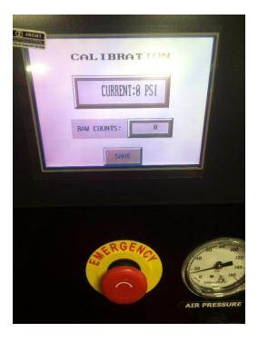
Once in the Calibration Screen, notice the raw counts and the current PSI. The current PSI should read 0 on a correctly zeroed tester. The counts are the unit of measurement read by the tester from the pressure transducer. If the tester hypothetically said 120 psi and 15 counts, the machine will need to be adjusted to read 0 psi and 0 counts. Steps 6 and 7 go along with step 5.
