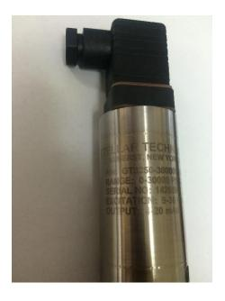
The Model # and serial # are located on the barrel of the pressure transducer.
