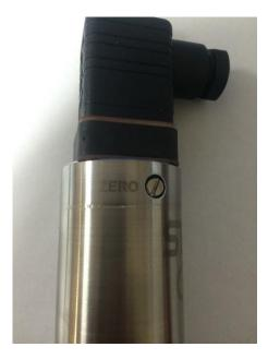
The trimmer on the pressure transducer will need to be reached in order to re zero the unit.
