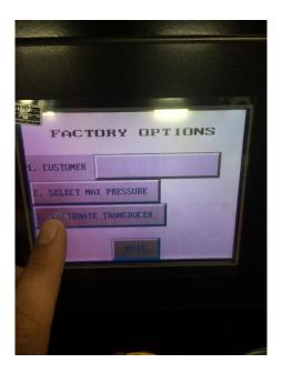
Select the "CALIBRATE TRANSDUCER" option on the visible Factory Options page.
