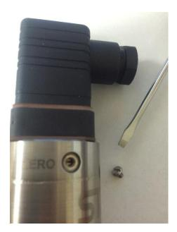
The cover screw will need to be removed. Underneath of this cover screw is a small set screw "trimmer pot". This is the screw that will need to be adjusted. Turning the screw Clockwise and Counterclockwise should produce a change to the counts and psi readings on the screen.
